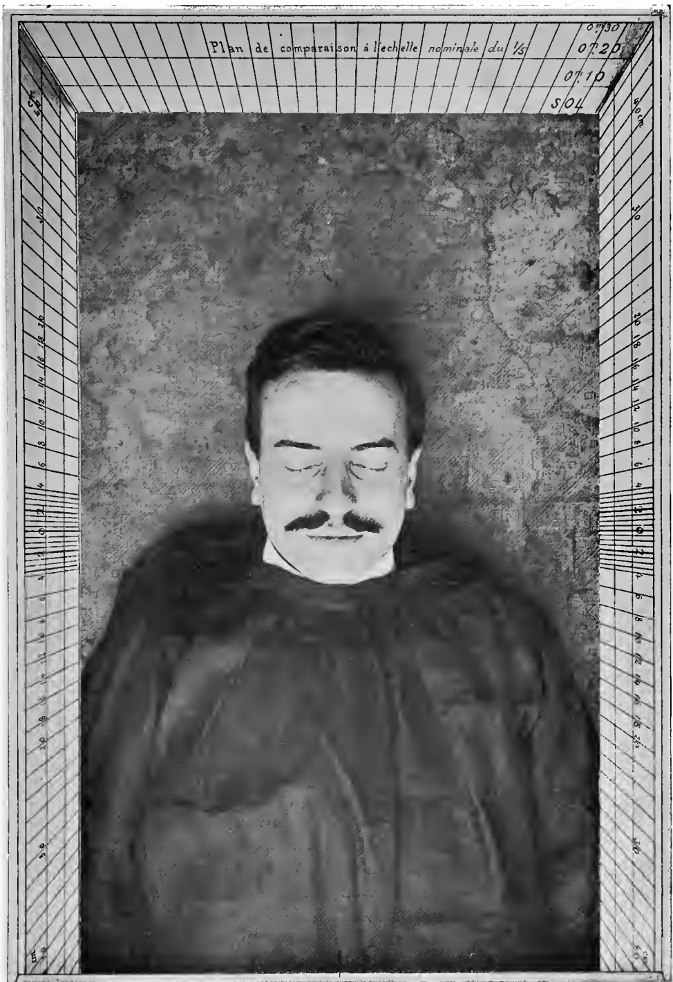
FIG. 7. — Perspectometric photograph at about \frac{1}{5} th reduction. Height of objective 9 metres, focal range 40 centimètres, perspectometric frame perpendicular to the ground of a relief of 30 centimètres, divided into horizontal planes of 10 centimètres equidistant, with gradations giving the corresponding value of the centimetre. To ascertain the depth, place the eye at 40 centimètres from the image opposite the middle of the line O O.
